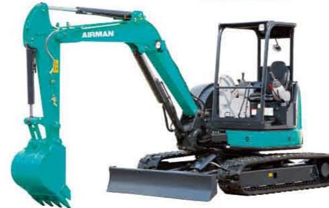
AX48U-6A Operating weight 4,540kg Capacity 0.14m 3 Rubber shoes, 4-pole canopy
