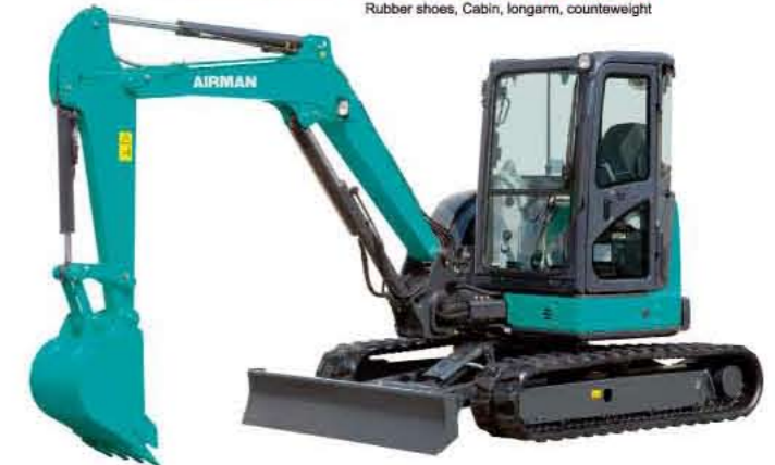
AX55U-6A Operating weight 5,210kg Capacity 0.14m 3 Rubber shoes, Cabin, longarm, countweight
