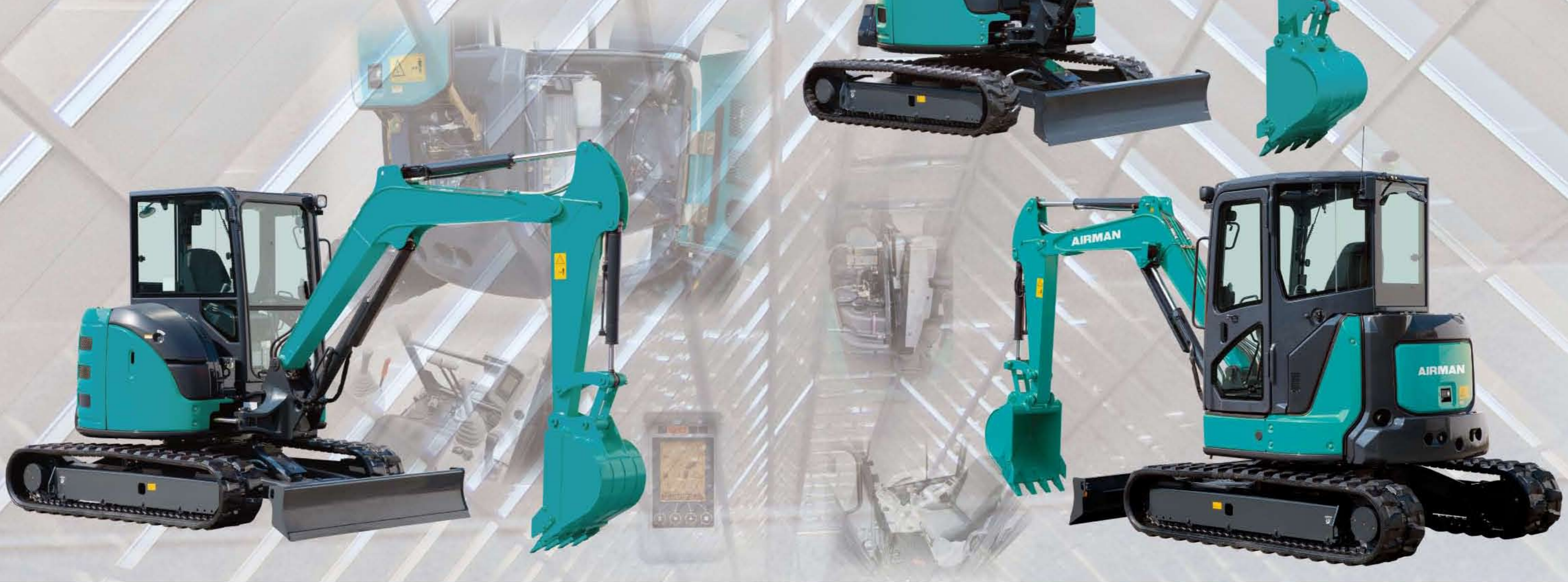
AX33U-6A Operating weight 3,130kg Capacity 0.09m 3 Rubber shoes, 4-pole canopy
